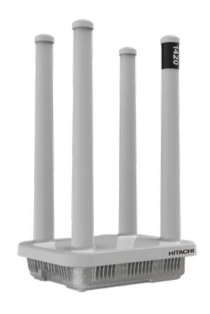
The TropOS 1420 provides superior reliability by accessing 653 MHz of RF spectrum (463 MHz in ETSI) using automatic interference avoidance capabilities of TropOS Mesh OS. It uses the 802.11a/b/g/n wireless standards to deliver 600 Mbps total wireless data rate, 300 Mbps at 2.4 GHz and another 300 Mbps at 5 GHz.
