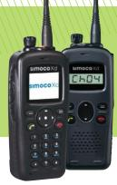
Available for DMR Tier II conventional, DMR Tier III trunked and analog modes of operation, Simoco Xd portables offer radio communication including intelligent Man Down, Lone Worker and full compliance with ETSI DMR standards.
